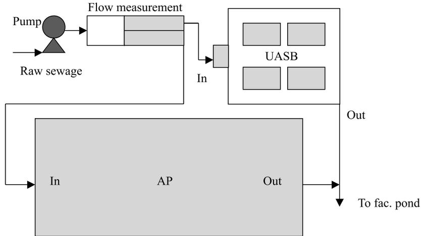
**Figure 1** Reactor layout and sampling point location
