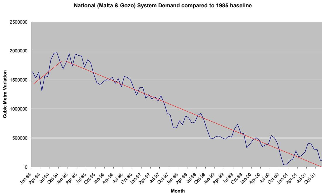
The above graph summarizes the effect of an aggressive national leakage control campaign. The graph depicts water produced and consumed, compared to a base year (1985) in order to eliminate seasonal fluctuations. Since water consumed consists of two components, legitimate consumer usage and leakage, a steady reduction in leakage has dropped production figures to practically pre-1985 values.
