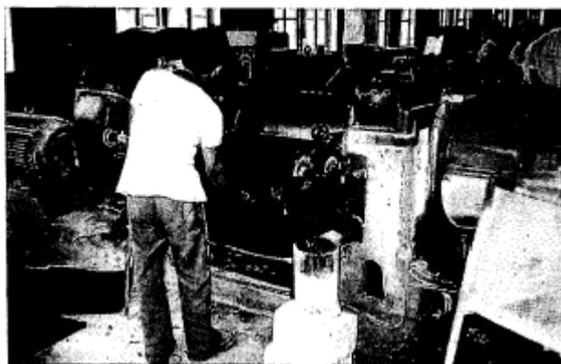
**Figure 4.4. The Devulcanized Rubber is Refined on a Calendering Machine, Shanghai, China.**
