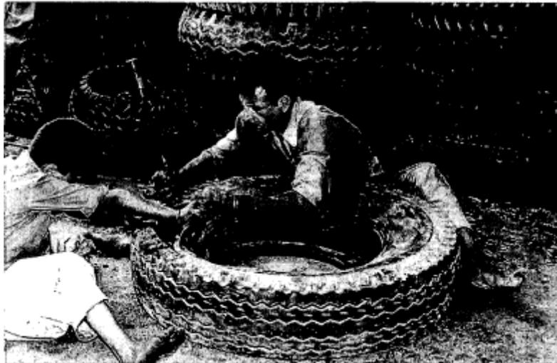
**Figure 3.10. Manual Separation of the Tread from the Sidewalls, Karachi, Pakistan.**
