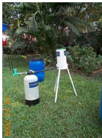
Figure 6: Tetrahedron Ion Exchange Resin Filter
