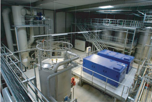
**Figure 2** Partial view of Seaborne plant with centrifuges and stripping column
